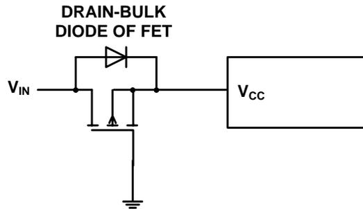
Figure 14. Low Loss Input Reverse Polarity Protection
