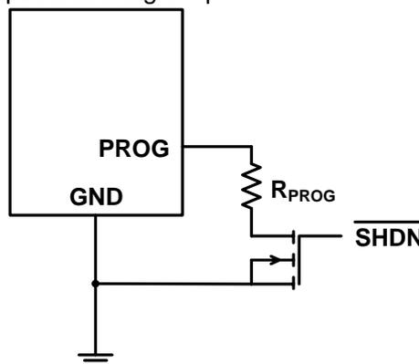
**Figure 6. Shutdown Operation**
