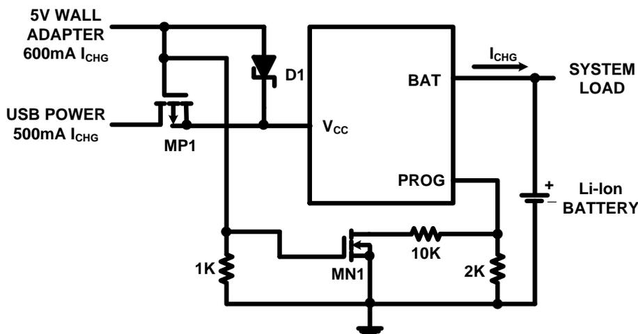
Figure 16. Combining Wall Adapter and USB Power
