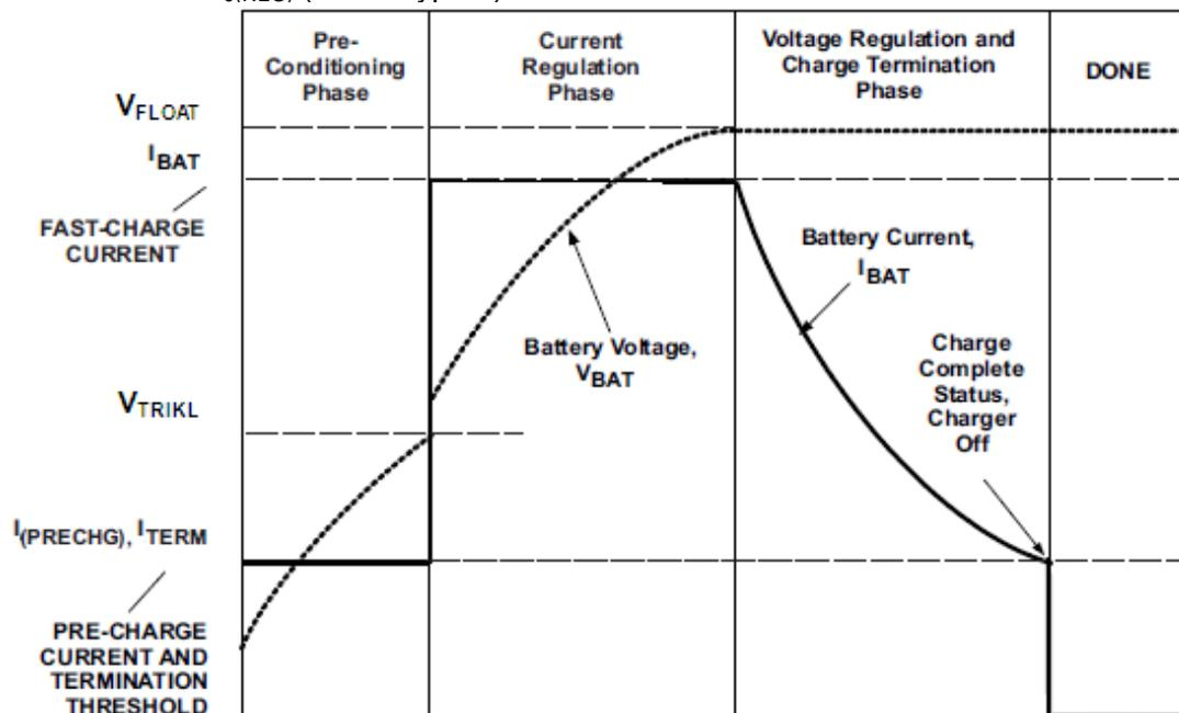
Figure 3. Charging Profile With  $T_{J(REG)}$
