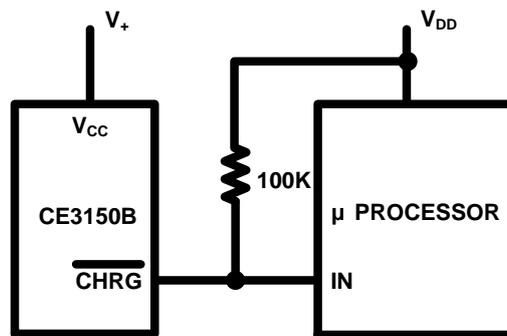
Figure 13. Using a Microprocessor to Determine CHRG State
