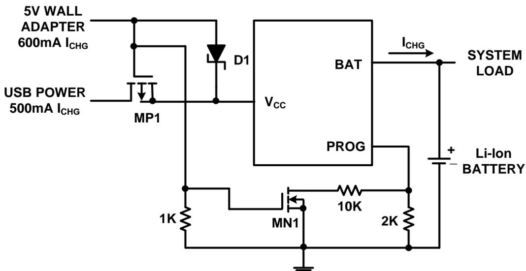
**Figure 11. Combining Wall Adapter and USB Power**
