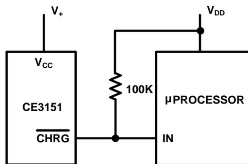
Figure 8. Using a Microprocessor to Determine CHRG State
