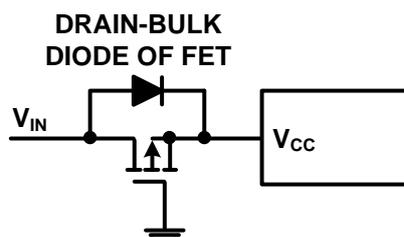
Figure 9. Low Loss Input Reverse Polarity Protection
