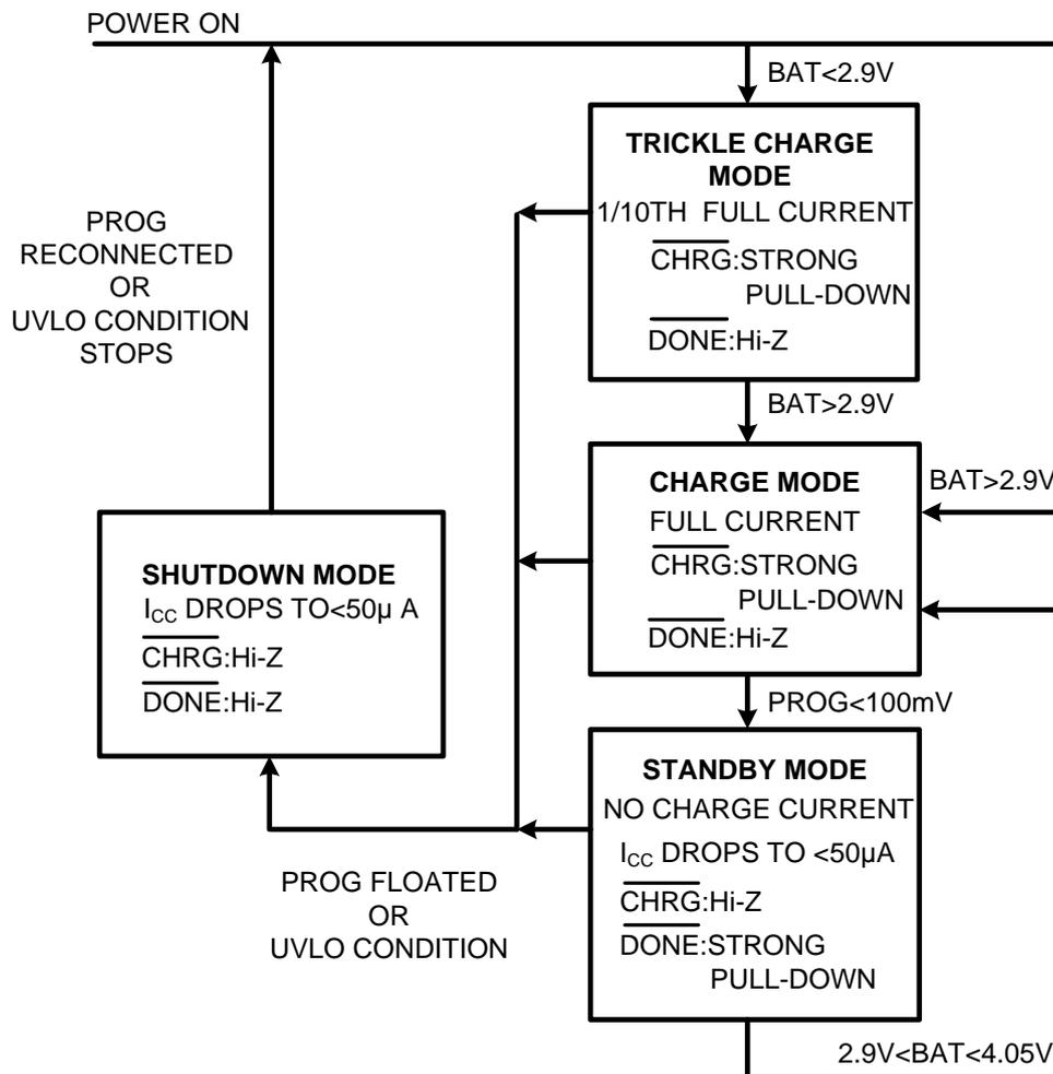
**Figure 3. State Diagram of a Typical Charge Cycle**
