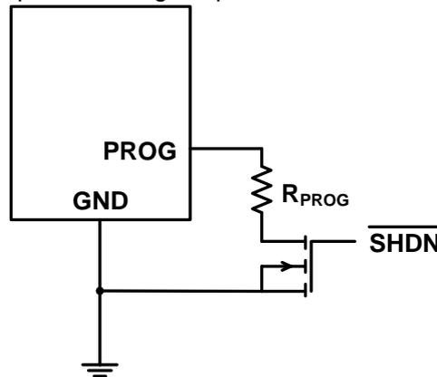
Figure 4. Shutdown Operation
