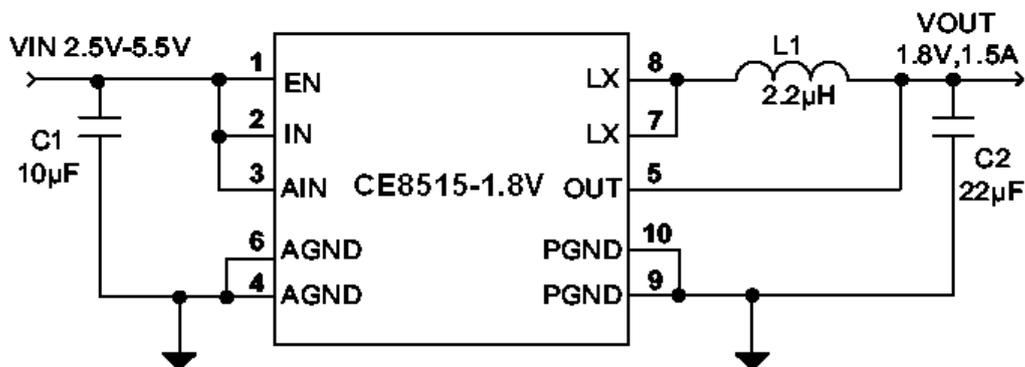
Figure3: Basic Application Circuit for the Fixed Output Versions.
