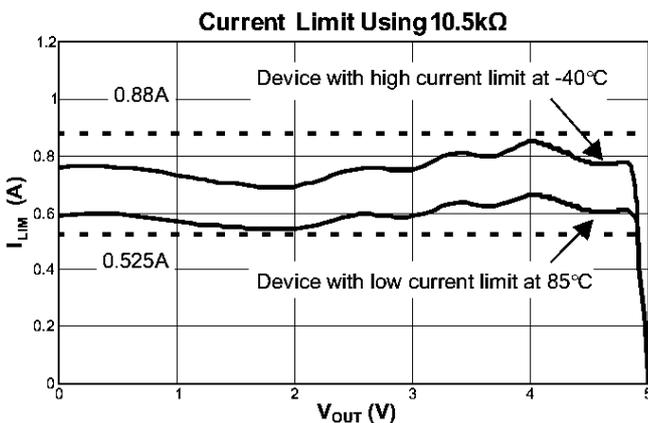
**Fig.1 Current Limit Using 10.5Kw**
