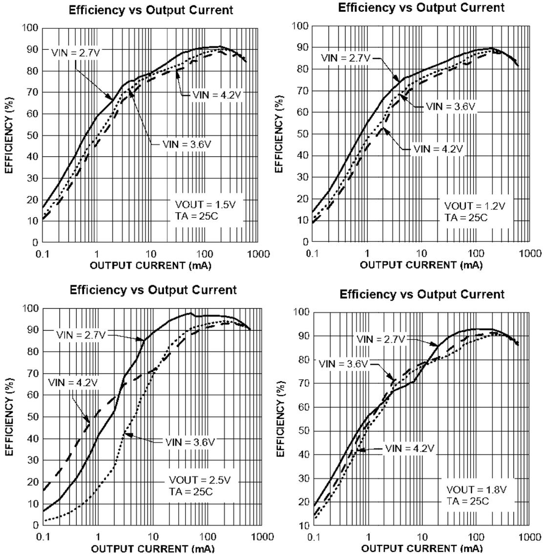
Efficiency vs Load Current
