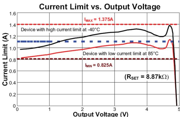
Fig.1 Current Limit Using 8.87k $\Omega$
