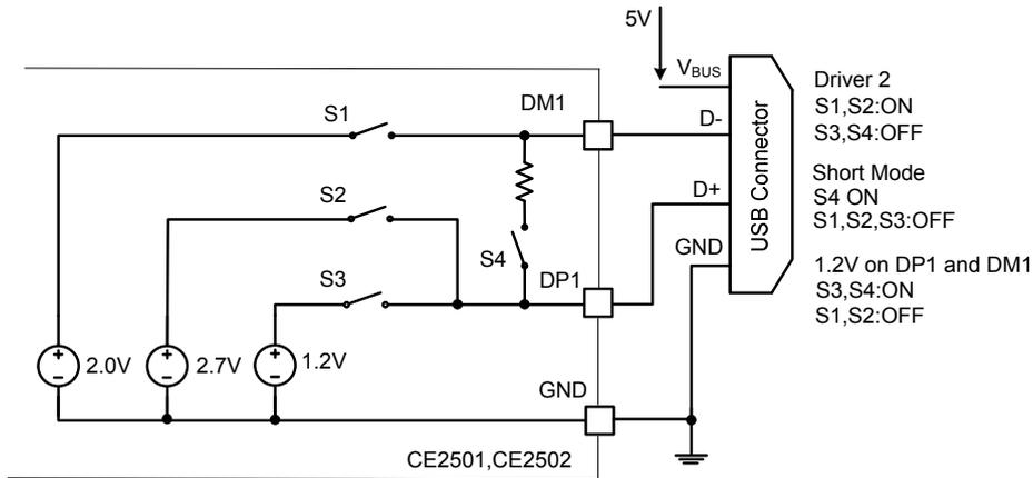
Figure 13. CE2501 and CE2502 DCP Smart-detect Function Diagram
