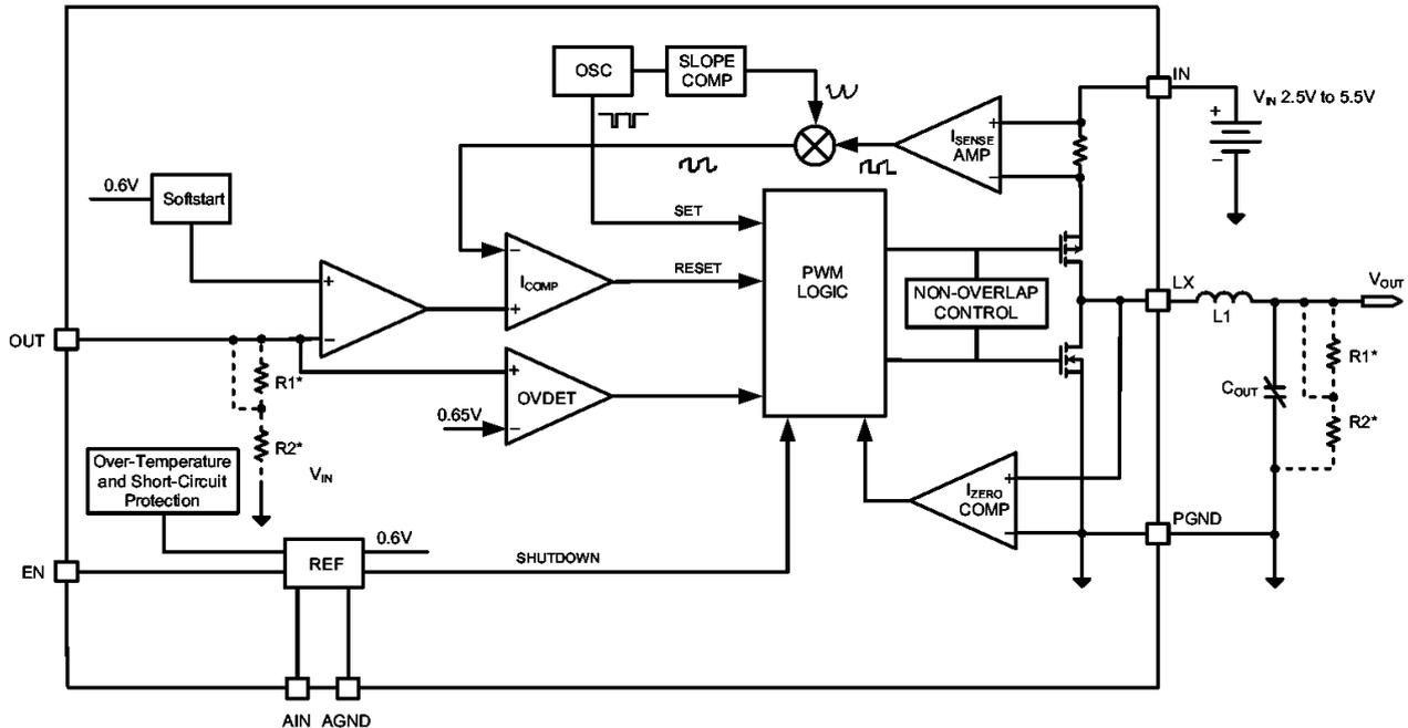
\*The resistor divider  $R1 + R2$  is internally set for the fixed output versions, and is externally set for the adjustable output versions.
