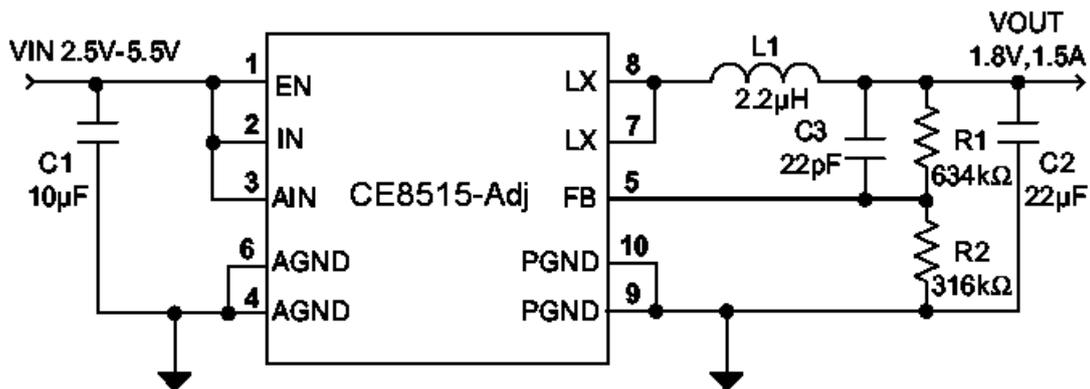
Figure2: Basic Application Circuit for the Adjustable Output Version.
