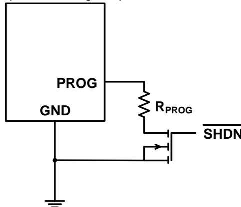
Figure 4. Shutdown Operation
