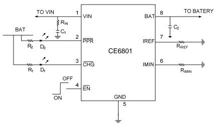
Figure1 Typical Application Circuit Interfacing to Indication LEDs
