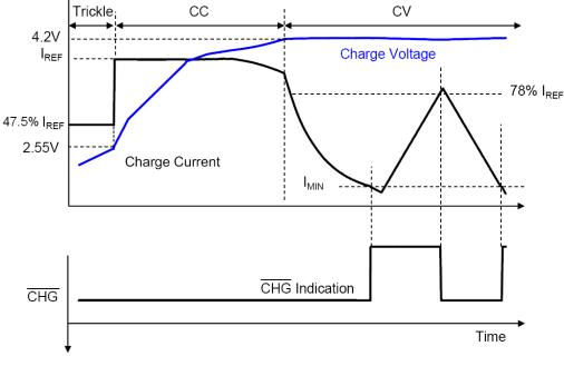
Figure3 Typical Charge Profile
